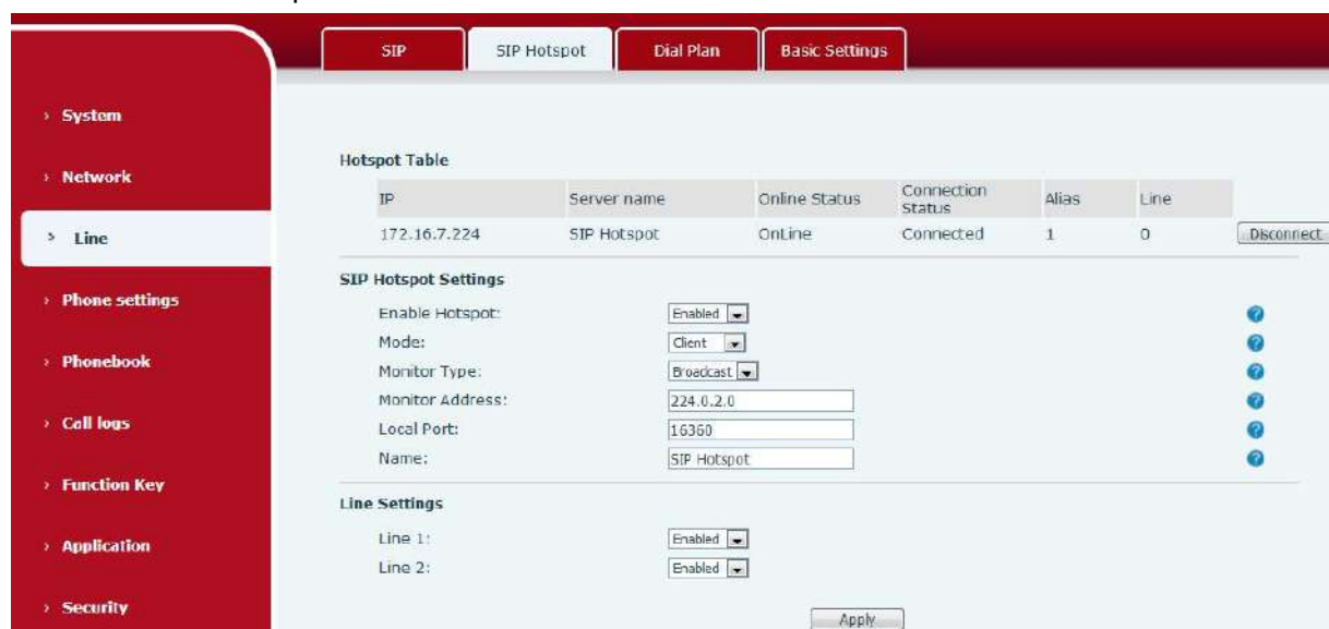
Picture 82 - SIP hotspot client configuration
