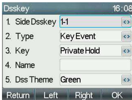
Picture 103 - DSS LCD key Page Configuration Screen
